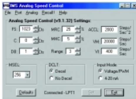
Figure 1.6.2: Speed Control Configuration Utility Screen
