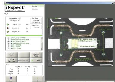
iInspect is a general purpose tool that includes capabilities for position control, measurements, identification and flaw detection. iLabel is a tool specifically designed for verifying the placement and quality of labels on packaged goods.
